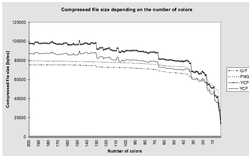
Figure 2. Compressed file size depending on the number of colors. Image: see figure 6.
