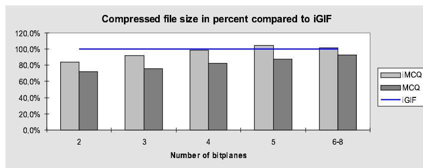
Figure 1. Compressed file size using iMCQ and MCQ compared to iGIF depending on the number of colors for the test image set (cf. table 1).
